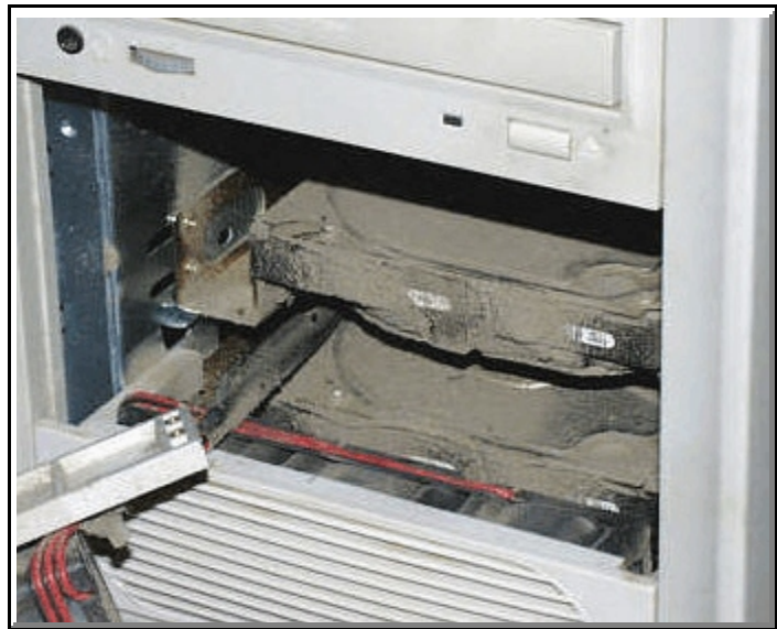
Dust accumulation on hard drives behind a drive-bay fan unit.
